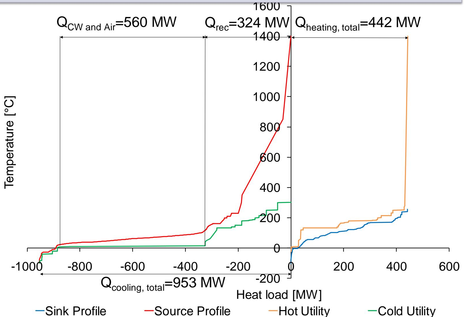
Step 3: investigate the potential to reuse heat from coolers as hot utility elsewhere. Total Site Approach (TSA)
